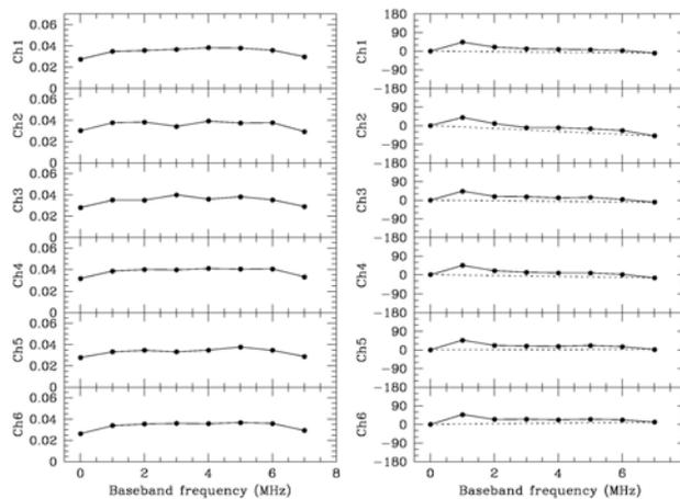
Phase shown after subtracting model ( $\text{phase}_{10\text{kHz}} + \text{delay} \cdot \text{freq} \cdot 360$ ), with delay = -0.19 us. Dashed straight line connects first and last phase points.
