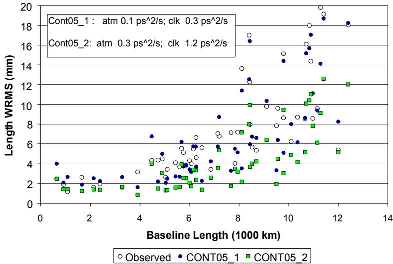
Figure. 1 Comparison of length repeatabilities observed during CONT05 and simulated.
