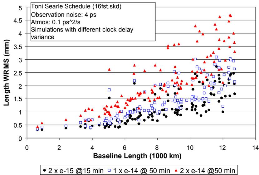
Figure 4. Sensitivity of length repeatability to clock variance. Random walk clock variances were varied from  $0.0036 \text{ ps}^2/\text{s}$  ( $2 \times 10^{-15}$  @ 15 min),  $0.3 \text{ ps}^2/\text{s}$  ( $10^{-14}$  @ 50 min), and  $1.2 \text{ ps}^2/\text{s}$  ( $2 \times 10^{-14}$  @ 50 min).
