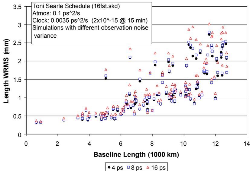
Figure 2. Sensitivity of baseline length repeatability to the observation noise ranging from 4 ps to 16 ps.
