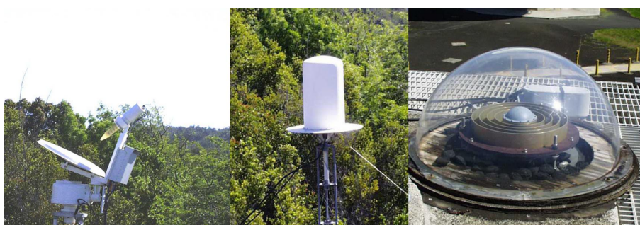
Figure 2. Kokee Park also hosts other systems; PRARE, DORIS Beacon, and IGS (Turbo-Rogue).
