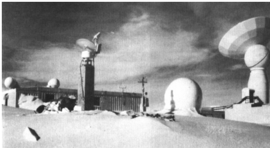
Figure 1. Geodetic Observatory O'Higgins – Antarctica : INMARSAT antennas at the station roof, PRARE Ground Unit (preliminary mounted in 1995), radome with GPS Turbo Rogue antenna and ERS/VLBI antenna. (October 1995)
