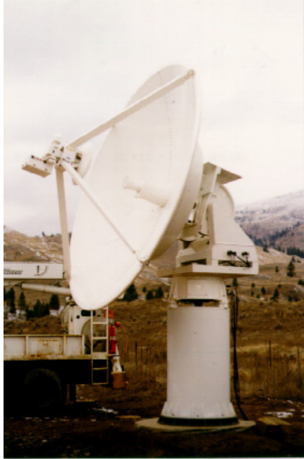
Figure 1. Canadian Transportable VLBI Antenna (CTVA)
