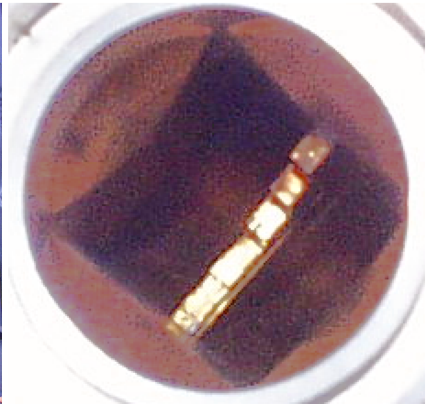
Figure 4: View into the COWAT showing the X-band septum polarizer sitting inside. The polarizer uses a stepped metal septum to separate the two modes into two rectangular waveguides for right hand and left hand circular polarization.
