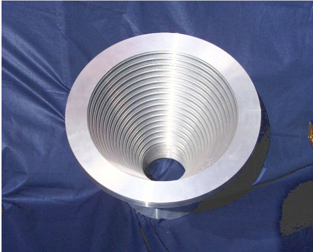
Figure 1: The dual-frequency corrugated horn.
