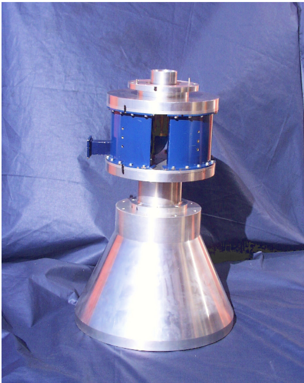
Figure 3: The feed horn and the COWAT mounted together.
