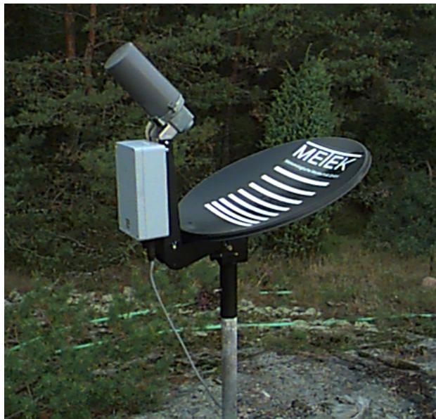
Figure 5: The zenith looking Micro Rain Radar (MRR) at the Onsala site.
