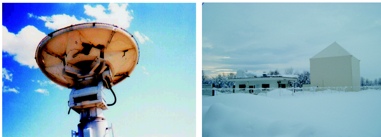
Figure 2. Left photo: Broken main reflector of SINTOTU3. Right photo: Antenna cover of SINTOTU3 for protecting the reflector from snowfall (Dec. 2001).
