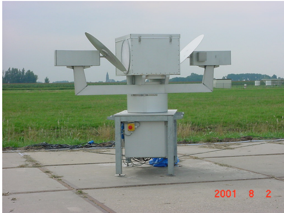
Figure 3. The new WVR operating at the KNMI test site in Cabauw in The Netherlands.
