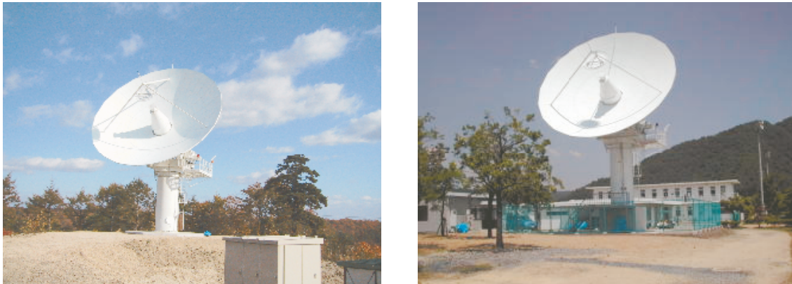
Figure 2. 11-m VLBI antennas at Tomakomai (Left) and Gifu (Right). These antennas and the VLBI observation facilities were transported from Miura and Tateyama KSP VLBI stations, respectively.
