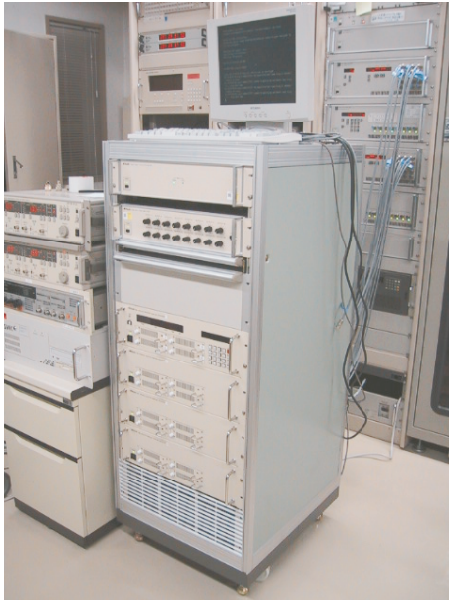
Figure 3. Full set of the K-5 VLBI observation system (Left) and 4-channel version for mobile observation (Right). The full set of the K-5 VLBI observation system consists of four PC systems with IP-VLBI board in each PC system.
