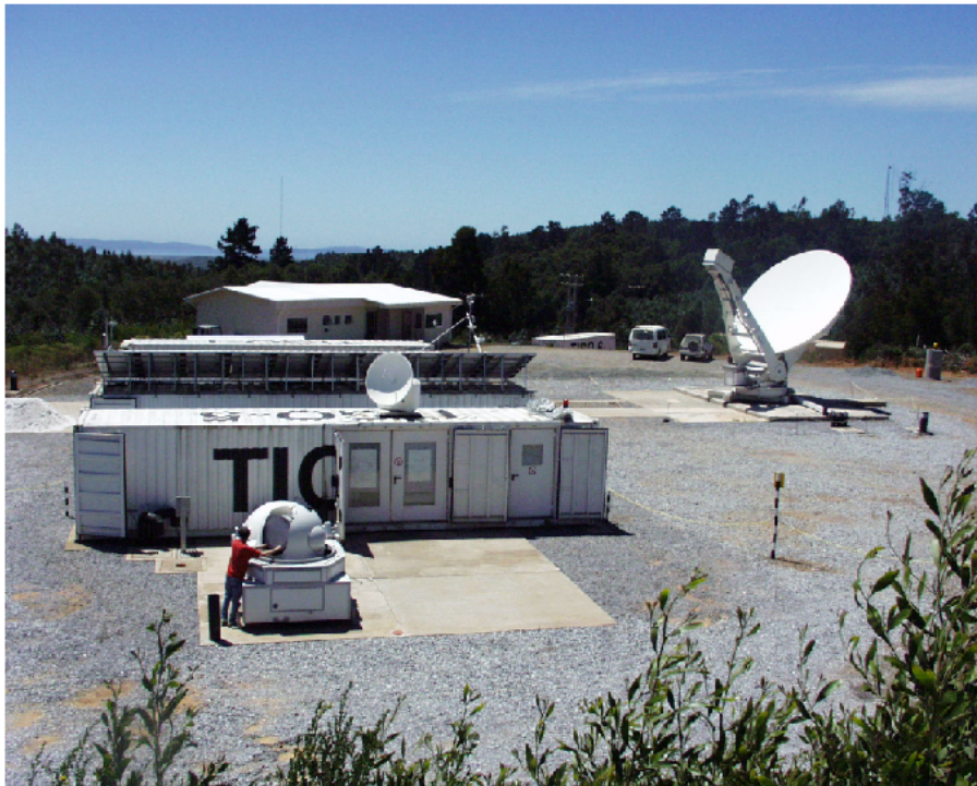
Figure 5. December 2002. The Geodetic Observatory TIGO is being installed and operational. In the foreground TIGO's SLR system, in the background TIGO's VLBI radiotelescope. Not in view is the GPS/Glonass IGS-Station which is in the back of the photographer. The Pacific Ocean can be seen at the horizon.
