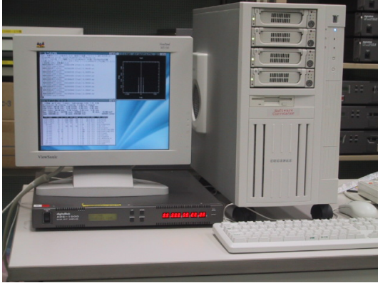
Figure 1. The PC-VLBI system: PC with PC-VSI board, display and a giga-bit A/D sampler (ADS1000). In PC-VLBI observation whole telescope IF sampling is accomplished by this combination.
