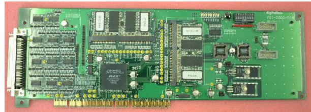
Figure 2. The PC-VSI data capture board. The 1024/2048Mbps VLBI data is transferred to PCI-bus continuously.
