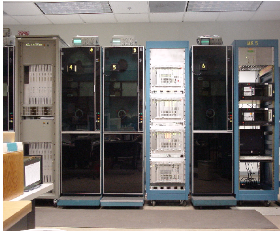
Figure 1. Partial view of Haystack Mark IV correlator, showing correlator rack, 3 tape units, 1 rack containing 4 SUs, and 1 rack containing 2 Mark 5A units and a decoder.
