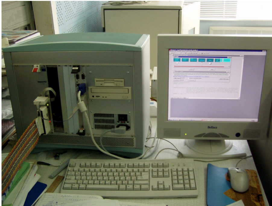
Figure 2. The prototype of Altera FPGA-based scalable correlator PARSEC with Mark4 specification.
