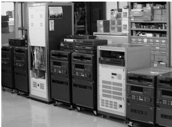
Figure 2. The Giga-bit VLBI system. The system in the left tall rack is GICO-I and that in the right short rack is GICO-II.
