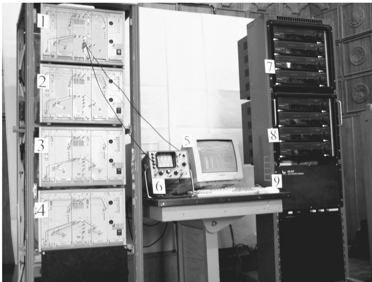
1, 2, 3, 4 — DAS modules; 5 — control PC; 6 — oscilloscope for phase calibration signal monitoring; 7, 8, 9 — S2-RT modules.
