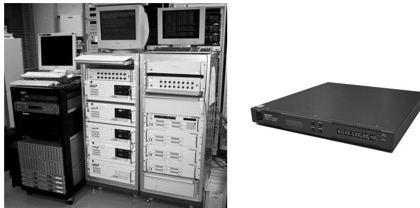
Figure 2. K5/VSSP VLBI system (right in the left panel) consists of 4 PCs. Each PC is equipped with one IP-sampler board, which has 4 channels of data input. Sampled data are recorded on their HDs as binary files. The maximum recording rate is 128 Mbps per PC. These recording PCs are also used for data processing purposes as correlators. K5/VSI VLBI system (left in the left panel) has capability of 1 Gbps recording rate per PC. Its data is fed from Giga-bits sampler (right) in VSI format.
