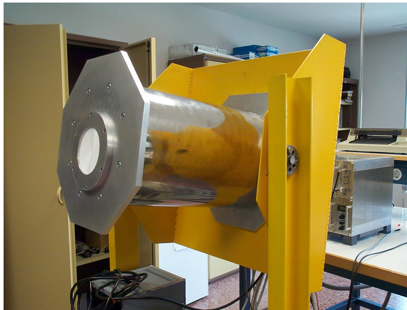
Figure 3. Cryostat of the 40-m telescope 22 GHz VLBI receiver.
