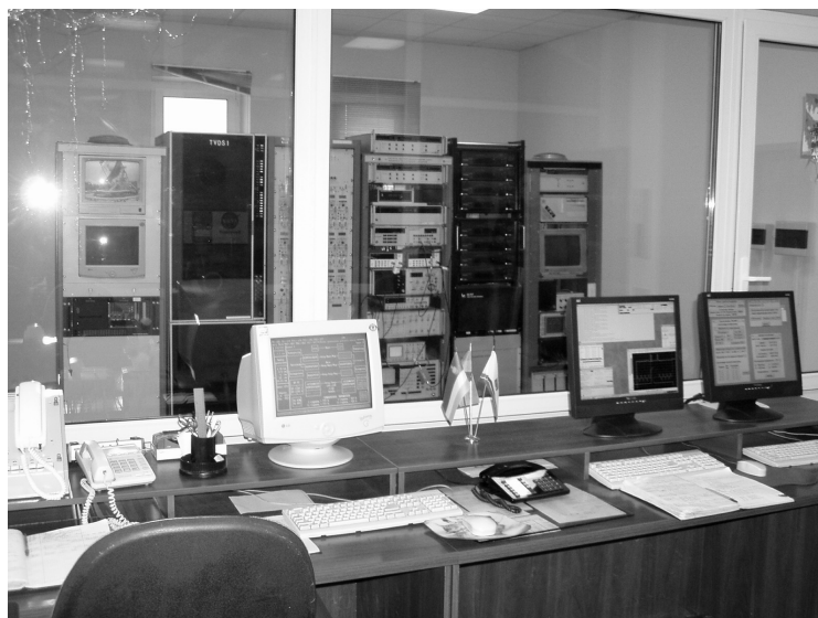
Figure 1. Upgraded control room of the radio telescope after installation of Mark 5 and S2-DAS systems.
