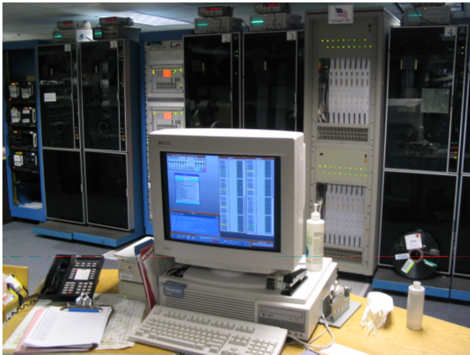
Figure 1. The left half of WACO showing 4 Mark 5A units (left), tape drives, the operator's console, and the central processor (right).
