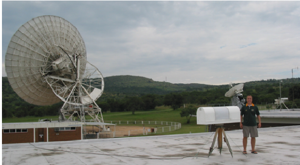
Figure 3. Attie Combrink inspects one of the water vapour radiometers on the roof of the main observatory building.
