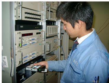
Figure 4. K5 sampling/recording system with hot-ejectable Serial ATA disks
