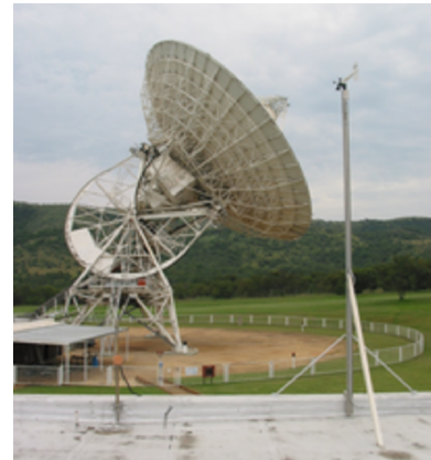
Figure 2. Anemometer on roof—the radio telescope is parked at zenith for 5 minutes when the wind speed exceeds 50 km/h.
