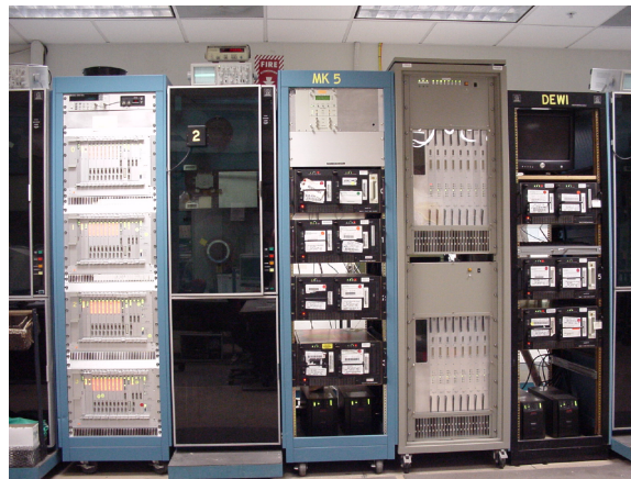
Figure 1. Partial view of the Haystack Mark IV correlator, showing 2 racks containing 7 Mark 5A units and a decoder, correlator rack, 1 tape unit, and 1 rack containing 4 Station Units.
