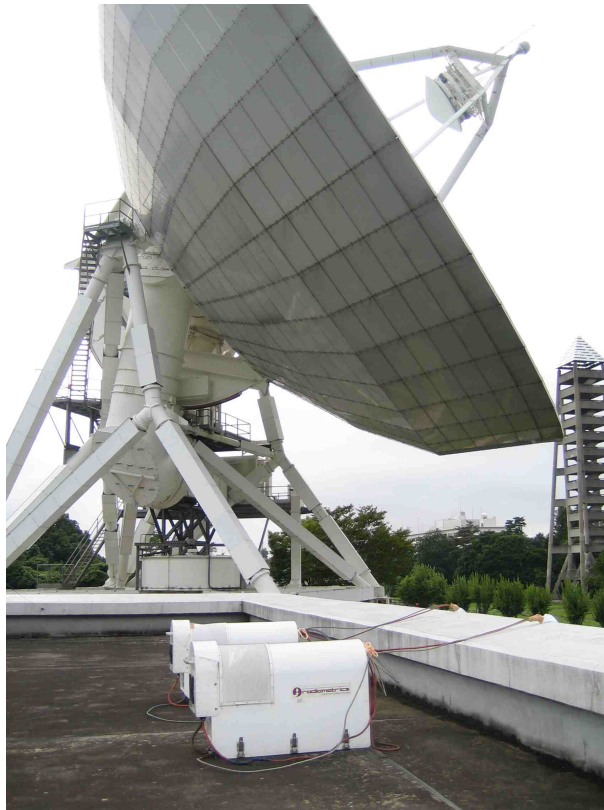
Figure 1. Two WVRs at the Tsukuba 32 m station of GSI. Both Kashima and Tsukuba were equipped with WVRs during the CONT05 campaign.
