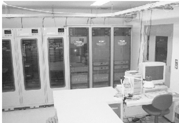
Figure 2. KSP Correlator room. The KSP hardware-correlation system, which has capability of 4 stations and 6 baselines of tape-based VLBI data processing.
