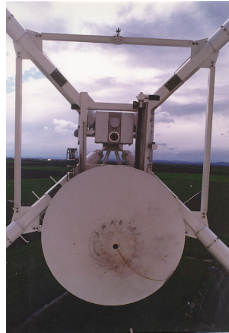
Figure 4. The primary focus receiver box and the subreflector.
