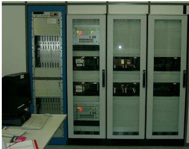
Figure 1. Left: Correlator rack in 2 crates. Middle: two station units with two rack-mounted Mark 5A playback units. Right: four Mark 5B units mounted in two racks.
