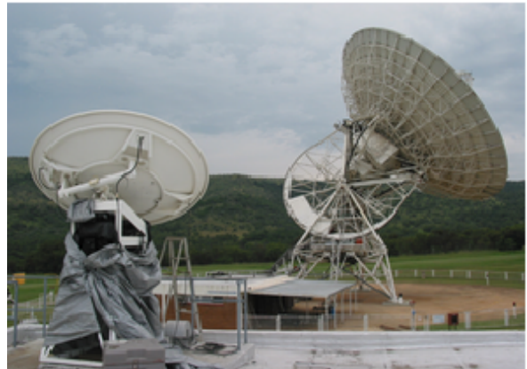
Figure 4. Holographic setup—reference antenna to collect 12 GHz signal transmitted from geostationary satellite.
