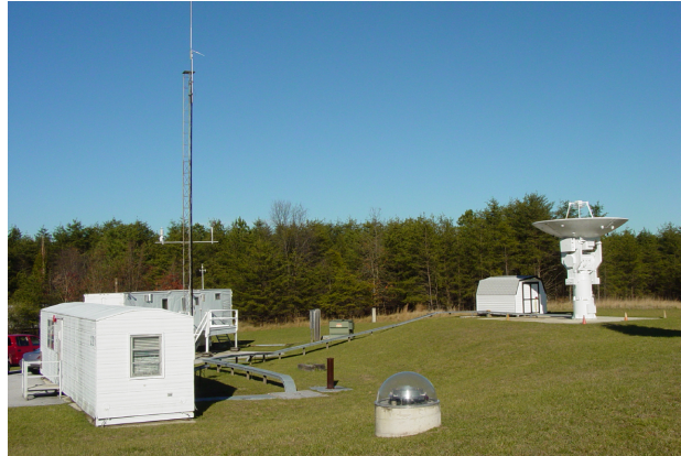
Figure 2. New permanent MV3 antenna.
