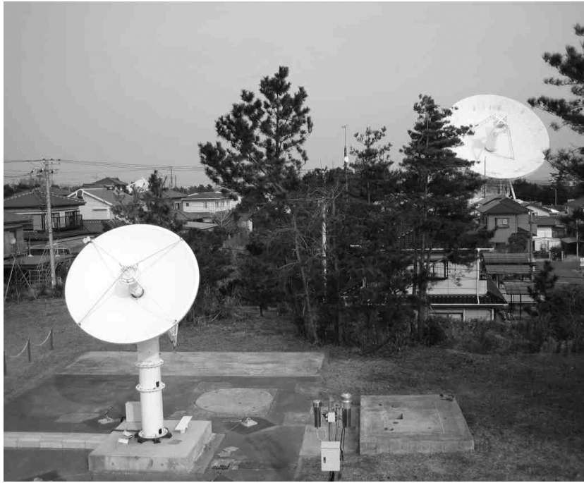
Figure 3. 2.4 m antenna (front) and 34 m antenna (back) at Kashima during a fringe test.
