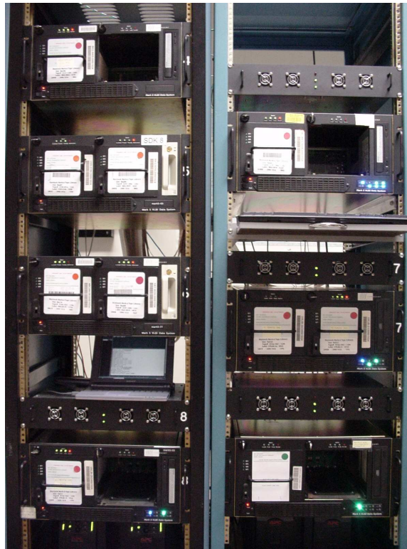
Figure 1. Partial view of the Haystack Mark IV correlator, showing 2 racks containing three Mark 5A correlator playback units, four Mark 5B DOM correlator playback units with associated correlator interface board units, and a laptop monitor.
