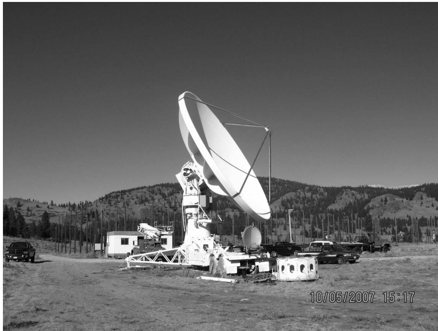
Figure 1. Ten meter prototype composite antenna at DRAO being prepared for holographic testing.
