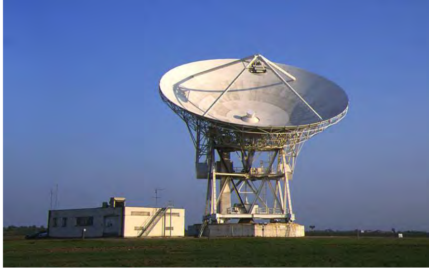
Figure 1. View of the Medicina 32 m dish taken during geodetic VLBI observations. Note that the subreflector is shifted to allow the use of the S/X receiver located in the primary focus of the radio telescope.
