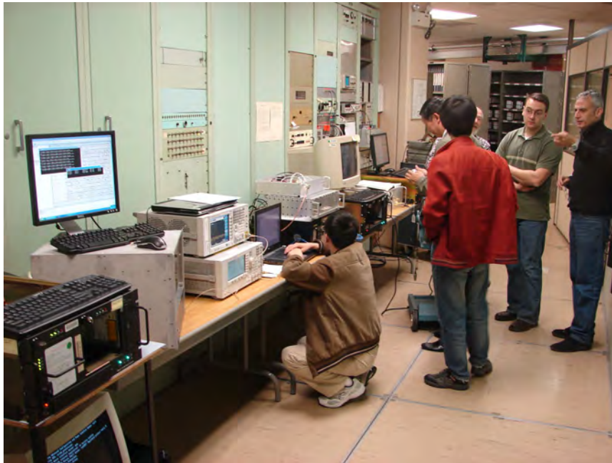
Figure 2. DBE intercomparison test setup at Haystack Observatory
