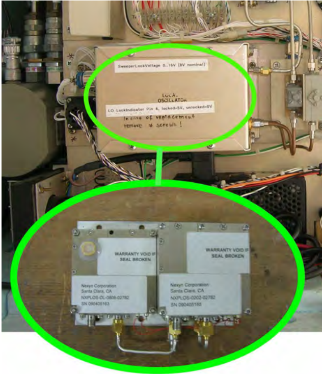
Figure 3. Replacement of the old Local Oscillator (upper circle) by the new LO (lower circle).
