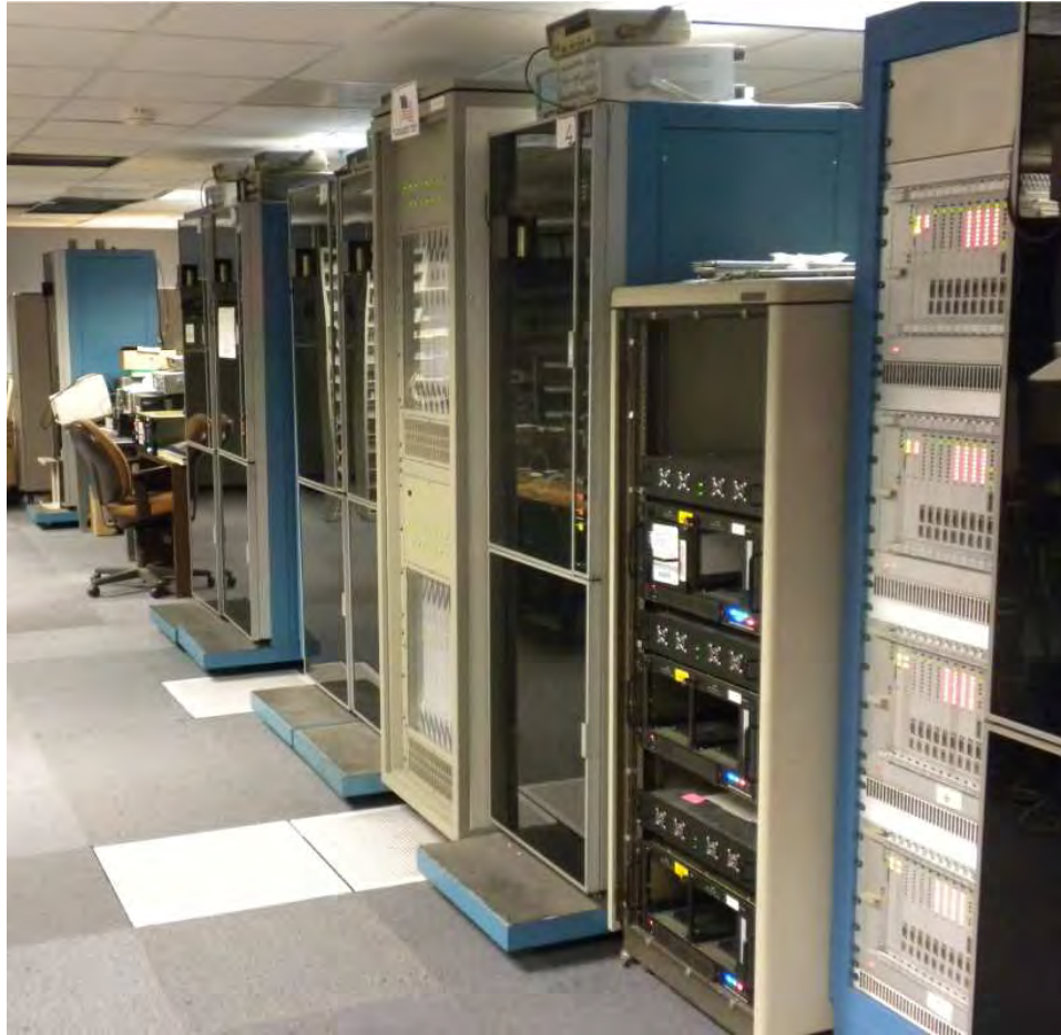
Figure 1. A view of the Mark IV Correlator. From right, station units, Mark 5B rack, legacy tape drive and central processing unit. More legacy tape drives are beyond the central unit. The Mark 5B+ in the background is used for e-VLBI transfers.
