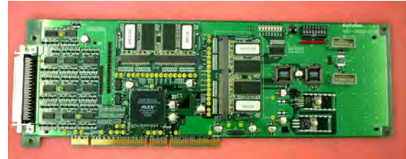
Figure 2. VSI-card can capture a high-rate data stream ( \leq 2 Gbps) through a VSI-H interface to a commodity PC.
