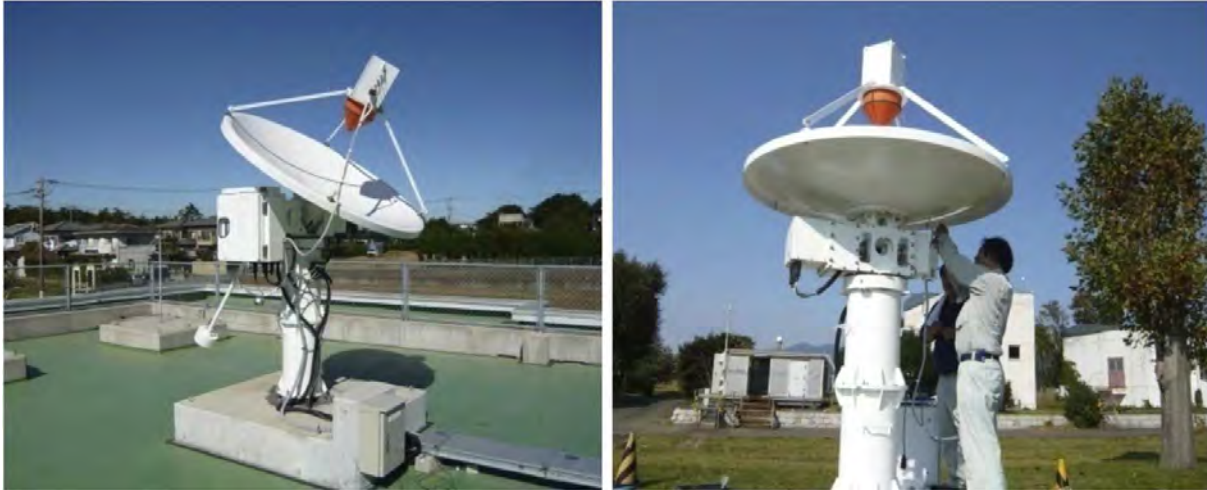
Figure 3. The MARBLE compact VLBI system. The left panel shows the first prototype at Kashima, NICT, and the right panel shows the second one at Tsukuba, GSI.
