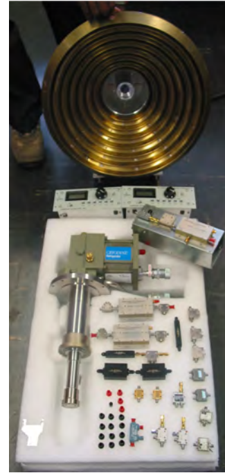
Figure 3. XDM feeds and receiver: prototype S-X feeds and components for the receiver. (Credit: R. Myataza)
