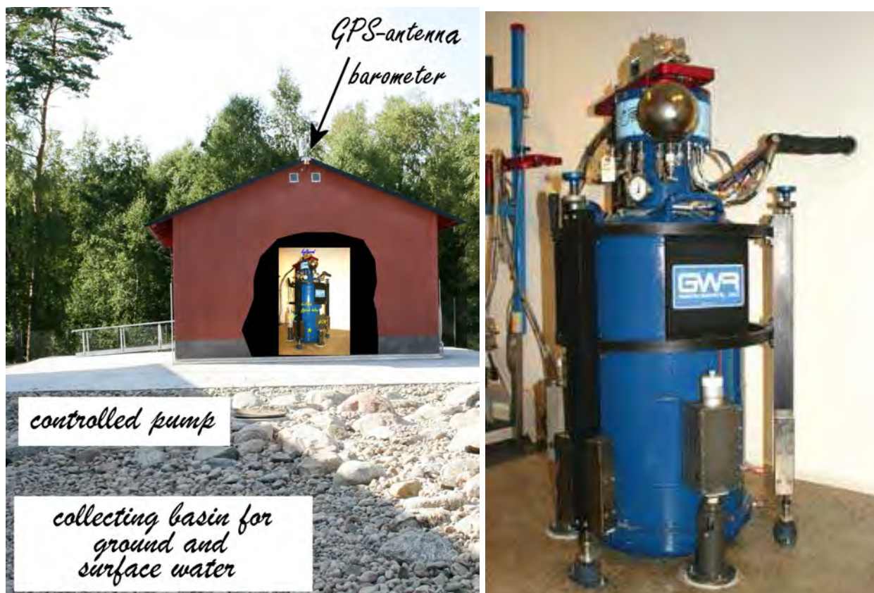
Figure 3. Left: The new gravimeter house at Onsala. Ground and surface water are collected, and the basin level is controlled by a pump. A barometer and a GPS time-receiver are located at the top of the new gravimeter house. Right: The new superconducting gravimeter “Hans” inside the gravimeter house.
