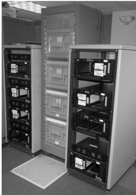
Figure 1. Conversion to Mark 5Bs: five Mark 5Bs (left rack and right bottom) share space with three Mark 5As (upper right) on the right side of the correlator. All of these will be Mark 5B by next year.
