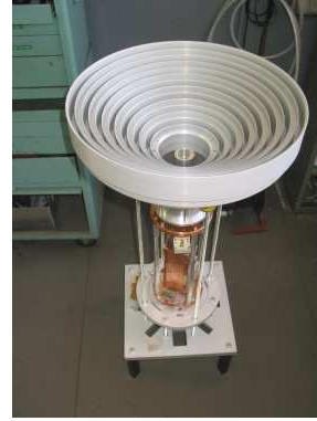
Figure 3. Test assembly of the XDM's S/X feeds and receiver.
