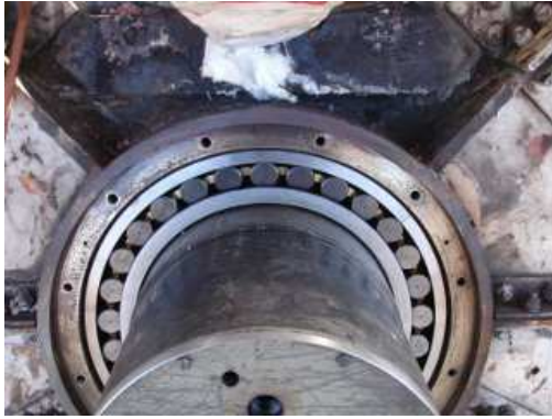
Figure 2. The new bearing is in place. (Credit: M. Gaylard)
