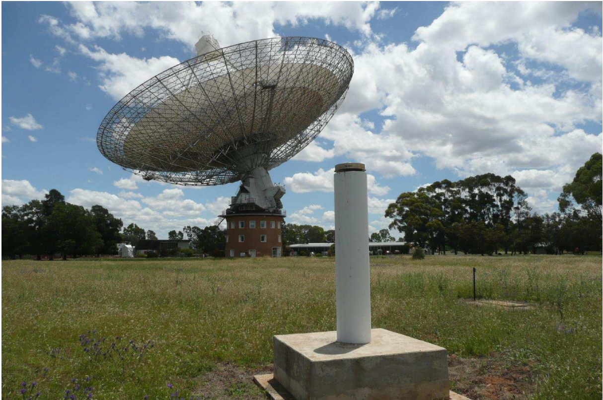
Figure 2. Parkes antenna, with geodetic monument and dual-frequency GPS antenna in the foreground. (Credit: John Sarkissian, CSIRO.)
