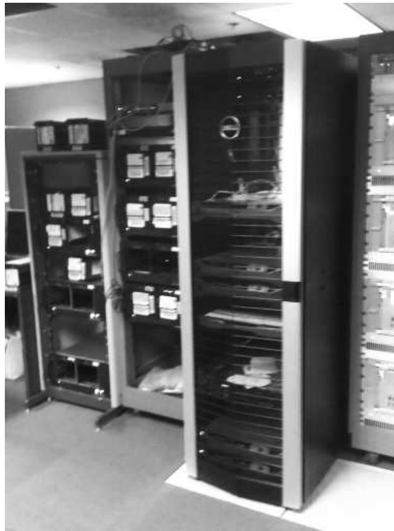
Figure 1. The e-transfer corner. A Storage Area Network (large unit) and three Mark 5B+s (far left) collect data over the high-speed networks and write the data out to Mark 5 diskpacks.
