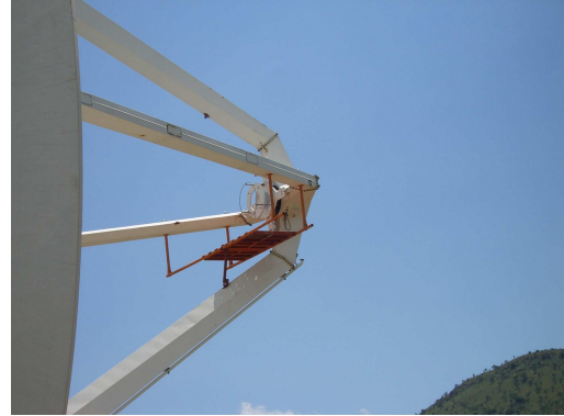
Figure 3. S/X receiver with integral feed to be installed at XDM prime focus. (Credit M. Nickola)
