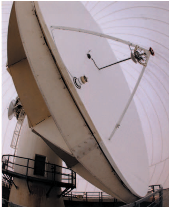
Figure 2. Wide-angle view of the Westford antenna inside the radome. The VLBI S/X receiver is located at the prime focus. The subreflector in front of the receiver is installed when observing with the TAL receiver (see Section 4), which is located at the Cassegrain focus.
