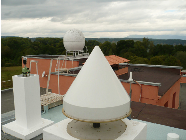
Figure 2. Javad GPS/GLONASS/Galileo receiver at the Zelenchukskaya observatory.
