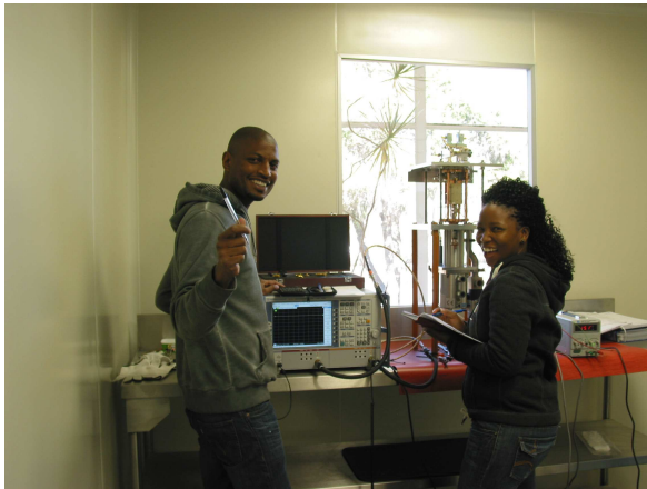
Fig. 2 Ronnie and Lerato in the microwave lab measuring T_{rec} of the 26 m's 3.5-cm Dicke switch cryogenically cooled receiver.
