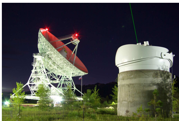
Fig. 2 Javad GPS/GLONASS/Galileo receiver and beacon “DORIS” at the Badary observatory.
