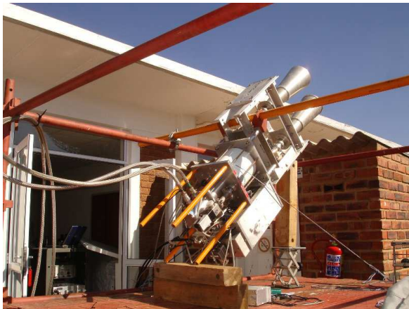
Fig. 3 T_{sys} measurements of the 26-m antenna's 3.5-cm Dicke switch cryogenically cooled receiver and feed.
