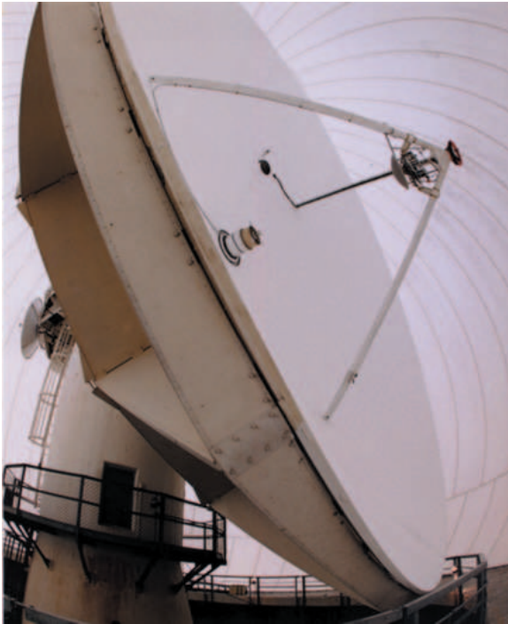
Fig. 2 Wide-angle view of the Westford antenna inside the radome. The VLBI S/X receiver is located at the prime focus. The subreflector in front of the receiver is installed when observing with the TAL receiver (see Section 4), which is located at the Cassegrain focus.
