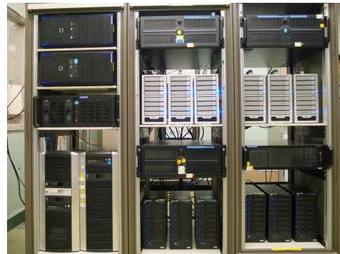
Fig. 1 The cluster computer of the correlator system using the GICO3 Software correlator at NICT/Kashima.
