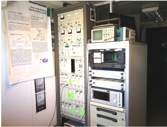
Fig. 3 The VLBA5 and Mk5B+ equipment used for VLBI observations of AGGO inside the AGGO-2 container.
