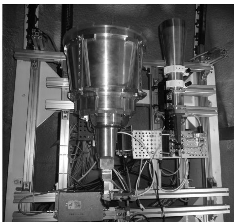
Fig. 2 A broadband NINJA feed has been installed in the receiver room of the Kashima 34-m telescope.
