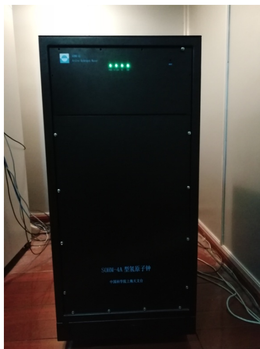
Fig. 4 The new on-site H-maser clock made at the Shanghai Astronomical Observatory.
