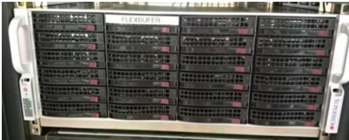
Fig. 3 The new Flexbuff hardware system at Tianma station.
