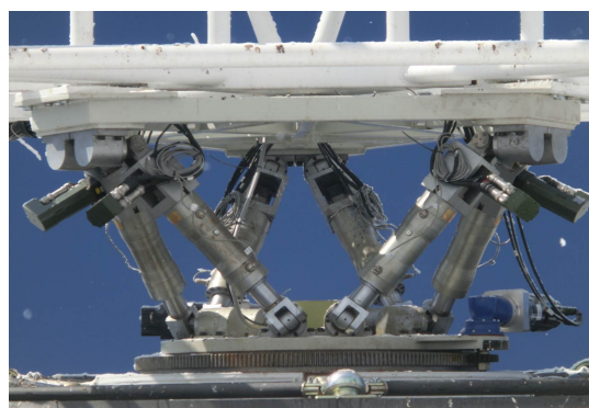
Fig. 2 The upgraded actuator motors on the Stewart platform of the NSRT.
