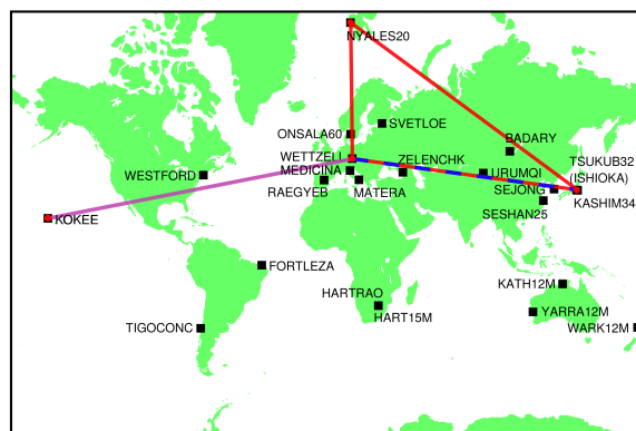
Fig. 2 VLBI stations mostly participating in IVS-R1 and -R4 sessions (black squares) as well as Intensives (red dots). INT1, INT2, and INT3 baseline vectors are plotted as purple, blue (dashed) and red lines, respectively.
