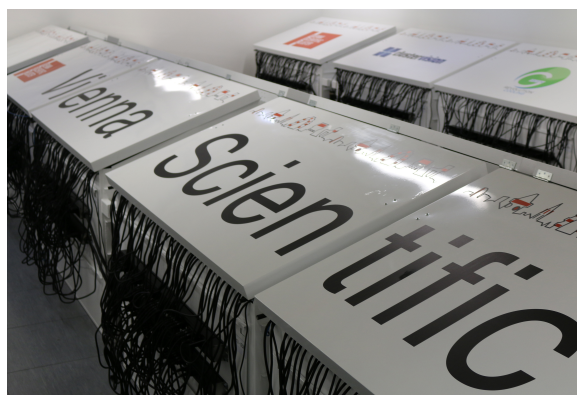
Fig. 1 Picture of the room where the 2020 nodes with liquid submersion cooling of the VSC-3 are stored. Picture was taken at VSC Arsenal TU Wien building ©Claudia Blaas-Schenner.
