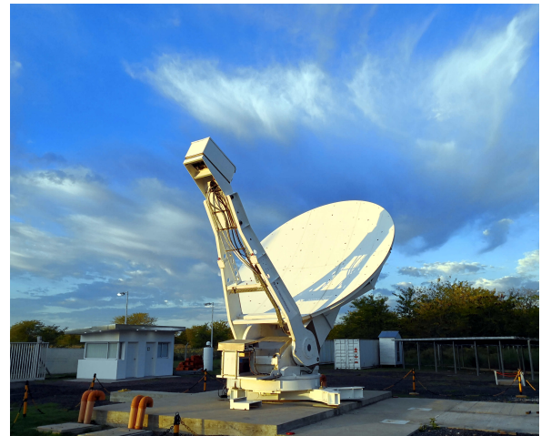
Fig. 1 The 6-m primary focus offset radio telescope for VLBI observations of AGGO.
