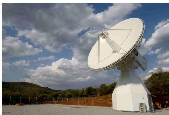
Fig. 2 The HartRAO VGOS radio telescope—mechanically functional but awaiting funding for receiver and backend.
