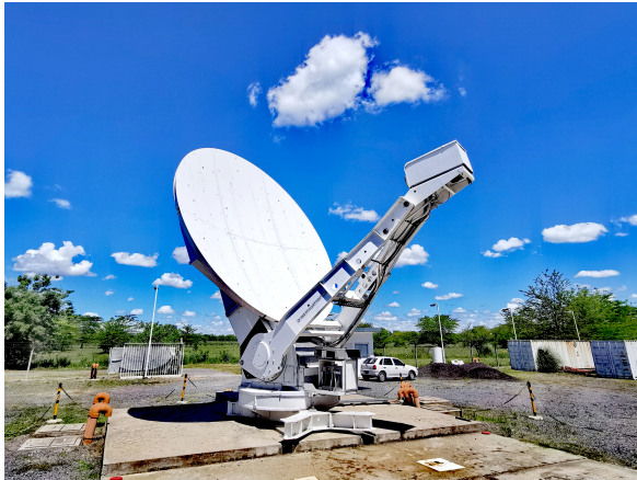
Fig. 1 The 6-m primary focus offset radio telescope for VLBI observations of AGGO became 25 years old in 2020.
