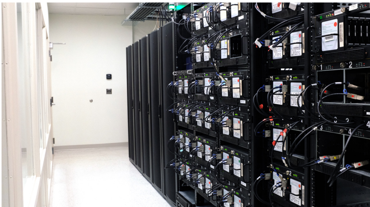
Fig. 1 Cluster correlator (background) and Mark 6 playback units (foreground) at the MIT Haystack Observatory.
