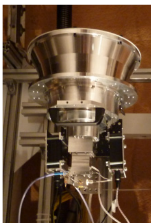
Fig. 2 Broadband ‘NINJA’ feed mounted on the Kashima 34-m antenna.
