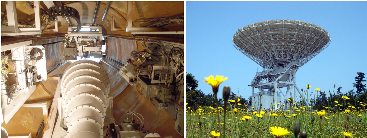
Fig. 3 Left: Bottom view of the Kashima 34-m antenna receiver room. Receivers are separated into four groups and mounted on one of four trolleys. Observing receiver is changed by exchanging the trolleys at the focal point (center). Right: The Kashima 34-m antenna and flowers.
