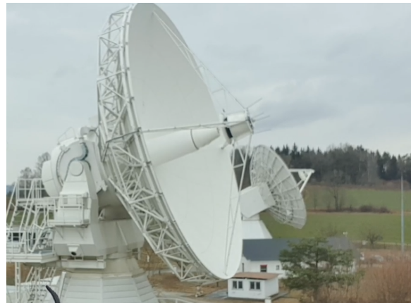
Fig. 1 View of the Geodetic Observatory Wettzell: in the foreground one of the two 13.2-m TWIN radio telescope antennas (Wn) and the 20-m Radio Telescope Wettzell (Wz) in the back.
