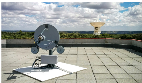
Fig. 6 Yebes RFI measurement system in the foreground and Yebes RAEGE VGOS radiotelescope in the background.
