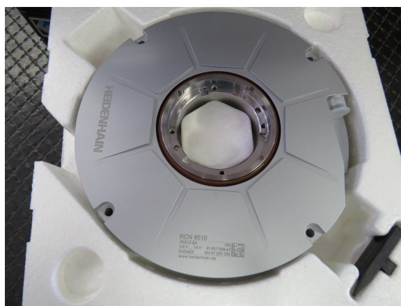
Fig. 4 One of the new HEIDENHAIN 26-bit absolute encoders awaiting installation after bearing replacement.
