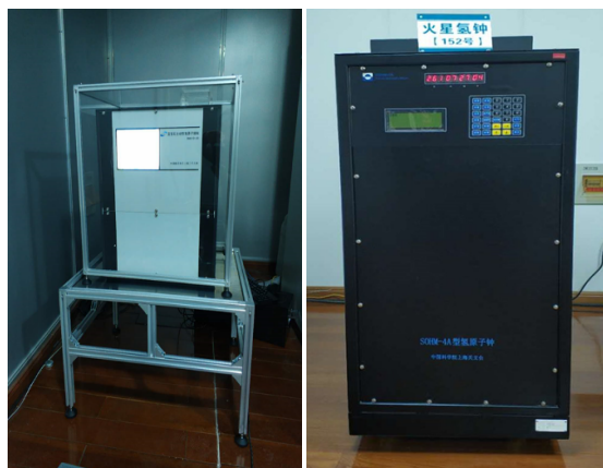
Fig. 5 Pictures of the hydrogen atomic clocks: (left) Domestic hydrogen clock 1, (right) Domestic hydrogen clock 2.
