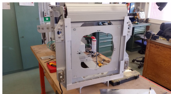
Fig. 3 RFI protection developed for the OTT receivers. The metal blinds can be activated from the VLBI field system to cover the feed horn and thus to protect against strong and potentially damaging RFI signals from, e.g., low earth orbiting radar satellites.
