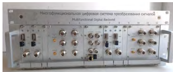
Fig. 3 The MDBE prototype for the RT-32 radio telescope.
