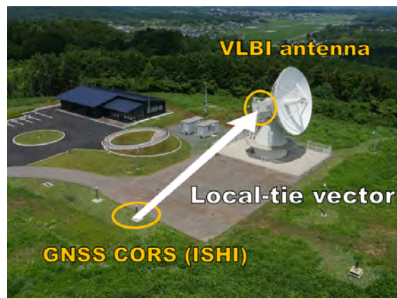
Fig. 3 VLBI-GNSS local-tie in Ishioka station.
