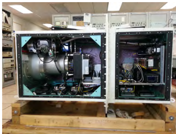
Fig. 3 20-m telescope VGOS Broadband Receiver.
