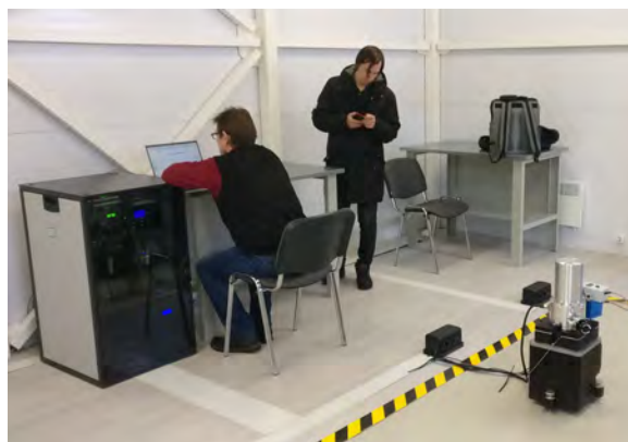
Fig. 2 Absolute ballistic gravimeter “LIAG-4” (bottom right corner) at Svetloe observatory.
