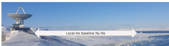
Fig. 4 The distance from the Ny telescope at Rabben to the Ns and Nn telescopes is about 1.5 km.
