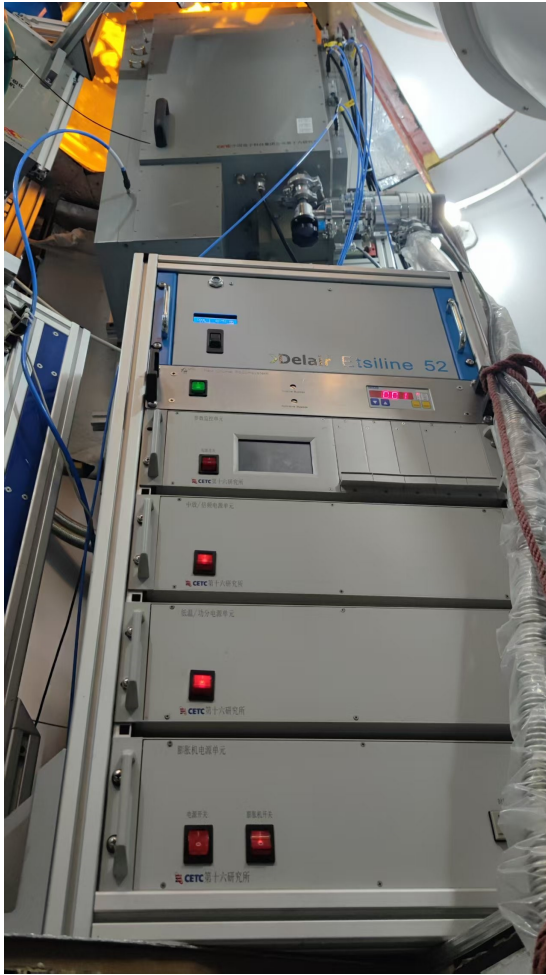
Fig. 2 Q-band receiver of the Nanshan 26-meter radio telescope.
