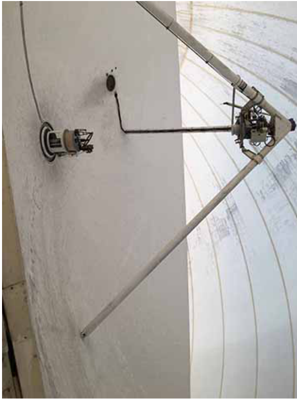
Fig. 2 View of the Westford antenna inside the radome. The VGOS broadband receiver is located at the prime focus.
