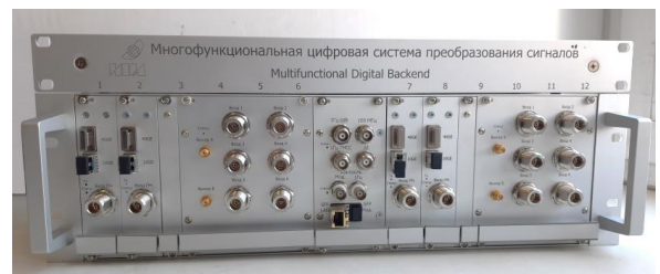
Fig. 8 MDBE for the RT-32 radio telescope.
