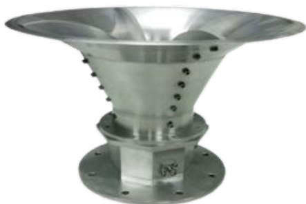
Fig. 2 Upgraded QRFH antenna.
