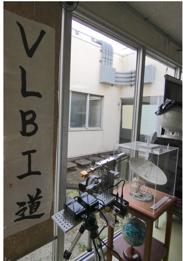
Fig. 1 Developed wideband feed and OMT for next generation radiometer at NICT Kashima.
