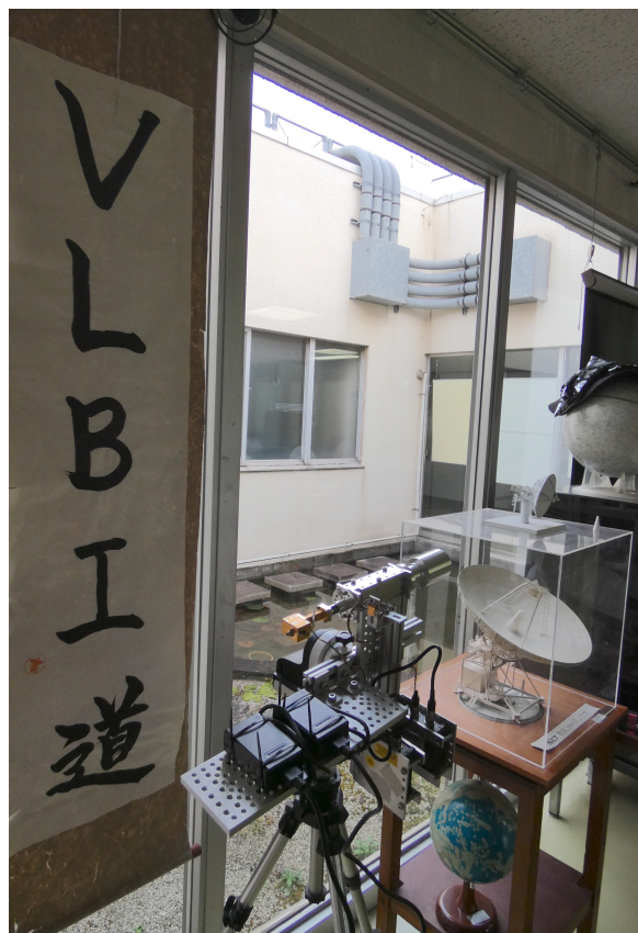
Fig. 1 Developed wideband feed and OMT for next generation radiometer at NICT Kashima.
