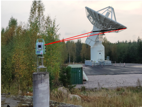
Fig. 1 Measurements with Leica TS50 robot tachymeter.
