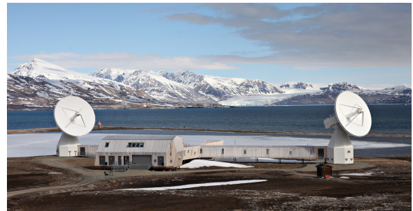
Fig. 2 The geodetic observatory's Brandal site with 13-m twin telescopes (Image: Bjorn-Owe Holmberg).
