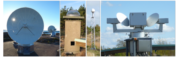
Fig. 2 Co-located instrumentation at the Onsala Space Observatory: The Onsala twin telescopes (left); ONSA and ONS1, two of the GNSS stations (middle); the microwave radiometer (right).
