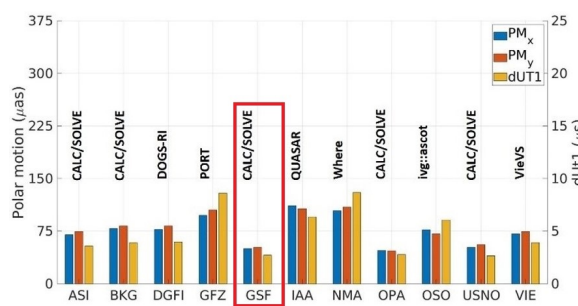
Fig. 5 WRMS of ERP estimation (AC minus Combination). Individual weights per AC are applied.
