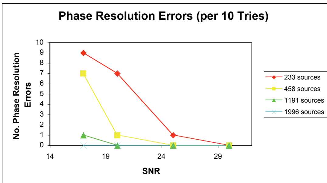
Fig. 4. Phase resolution errors (for 10 tries) vs. SNR for four sources, each having a
